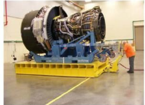
A General Electric GENX engine being handled with the HovAir technology at our Everett, Washington nacelle facility.
